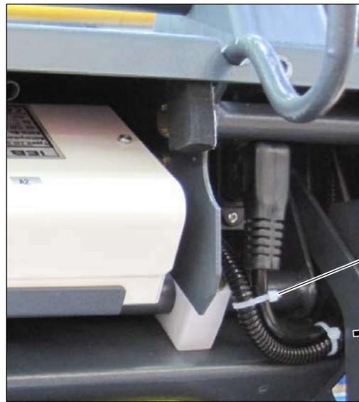
The cable from the handlebar switch must be fixed to the power aplug by cable ties.
